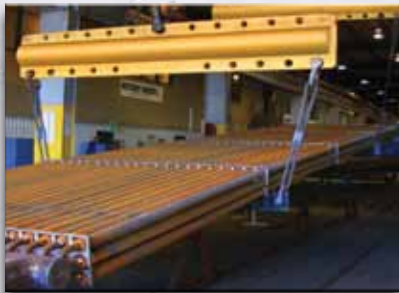
Modular HRSG tube bundle being prepared for internal inspection.
