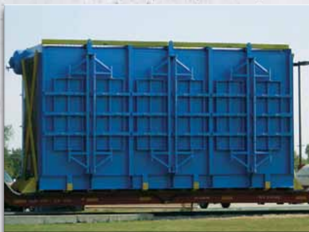
MSW boiler equipped with large Davit doors for easy access.
