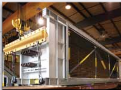
HRSG modules are designed for ease of lifting and movement.
