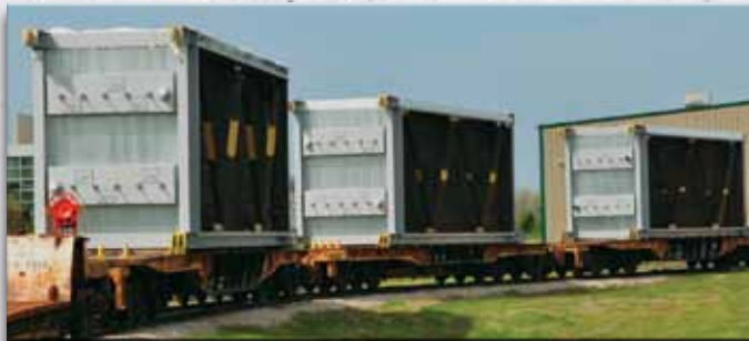
Three of six HRSG modules designed to ship by rail.
