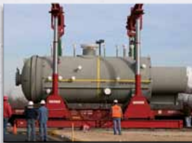
Victory Energy specializes in large-scale fabrication of boilers and pressure vessels.
