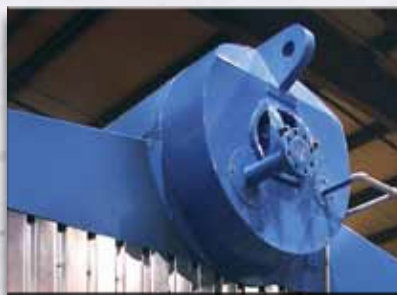
Drum heads are assembled with ceramic insulation covered with carbon steel.
