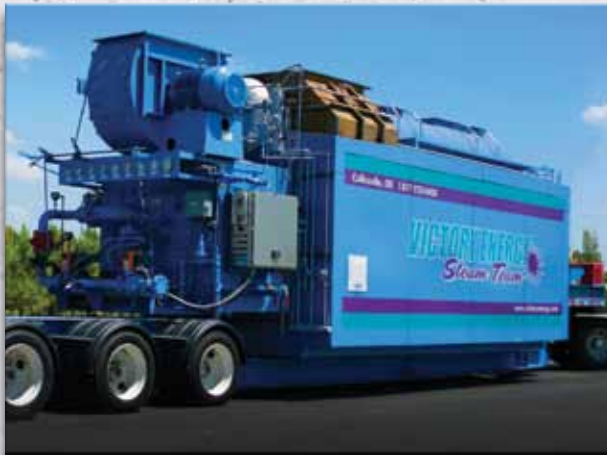
Fleet of Rental Boilers mounted on heavy-haul "Drop-N-Go" trailers.
